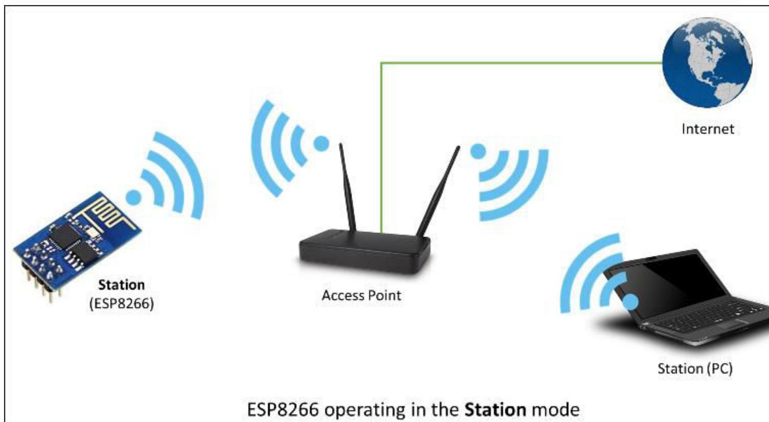
Station class has several features to facilitate management of Wi-Fi connection. In case the connection is lost, ESP8266 will automatically reconnect to the last used access point, once it is again available. The same happens on module reboot. This is possible since ESP is saving credentials to last used access point in flash (non-volatile) memory. Using the saved data ESP will also reconnect if sketch has been changed but code does not alter the Wi-Fi mode or credentials.
